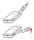
Before learning the device, the cover needs to be removed to expose the learn button and batteries. The device's case has 3 opening points; using a flat bladed screwdriver, carefully push into 1 of these points and prise open.
