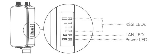
Device cable gland must be positioned vertically downwards to protect it against water ingress.
