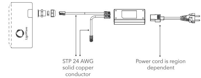
STP 24 AWG solid copper conductor
