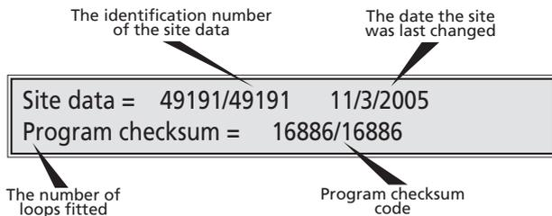
Matching site data codes, i.e. 49191/49191 and program checksum codes, i.e. 16886/16886, show that the panel is functioning correctly. Mis-matched numbers, i.e. 49191/40286, indicate that the panel's memory may be corrupt. After five seconds the panel will return to the Engineering Functions submenu.
