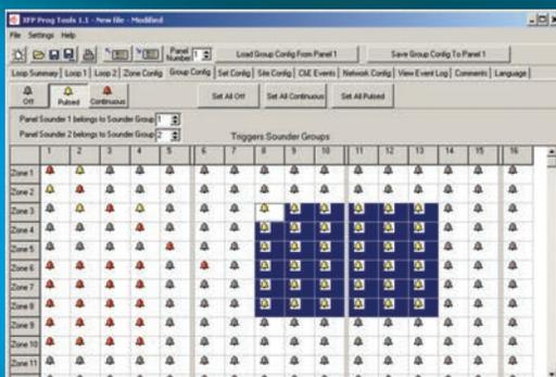
Sophisticated sounder group mapping (above) and complex cause and effect scenarios can be easily implemented using the XFP's intuitive upload-download programming software.
