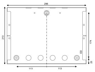
Mx-5010/Mx-5020 Enclosure Size and Fixing Point Dimensions
