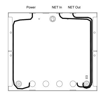
Internal arrangement showing recommended routing of cables.
