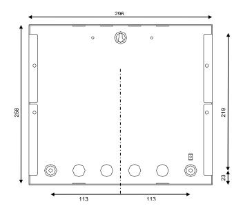
Mx-5030 Enclosure Size and Fixing Point Dimensions
